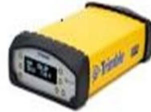
Figure 10- DGPS Survey Instrument
