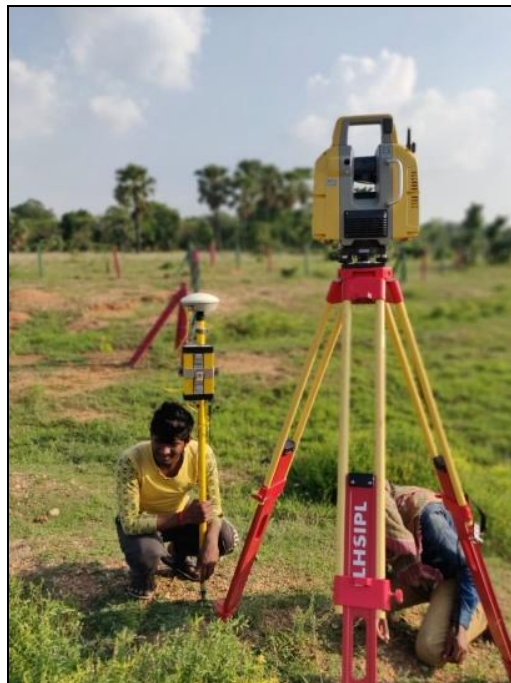
Figure 2- Topographical Survey with GLS 2000 3D Laser Scanner
